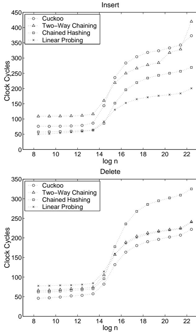
Fig. 4. The average time per update operation in equilibrium for load factor  $1/3$ .
