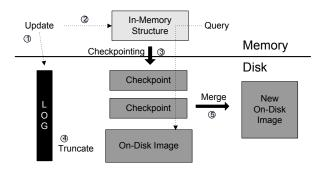
Figure 2: A Log-Based Storage System Architecture.
